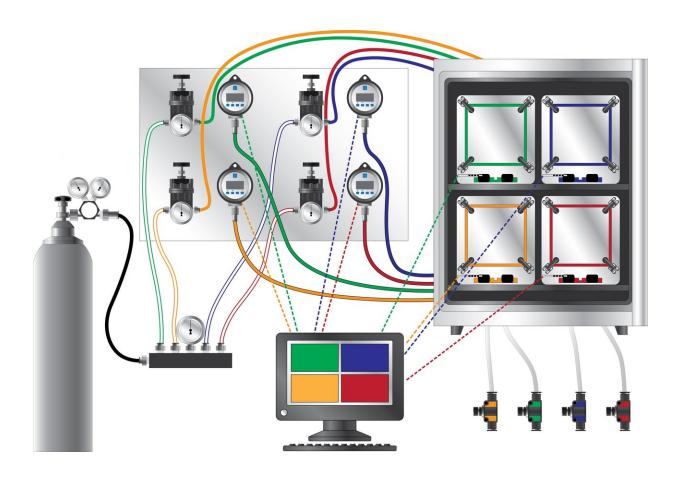
Housed inside a commercial cell culture incubator (A) are separate Plexiglas pressure chambers (B). Pressure is generated via compressed breathing air with 5% CO2that is controlled by a dual stage regulator (C) connected to manifold (D) which distributes the compressed air to separate pressure valves (E) that deliver compressed air to the pressure chambers. Flow rates are further controlled by pinch valves (G) connected to outflow lines. Pressure inside each
