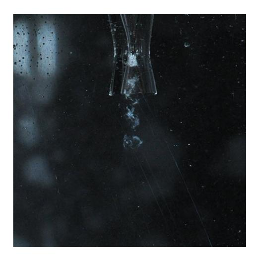
The researchers used a certain type of nozzle to create the cavitation bubbles which removed the plaque when they collapsed. Credit: Hitoshi Soyama
