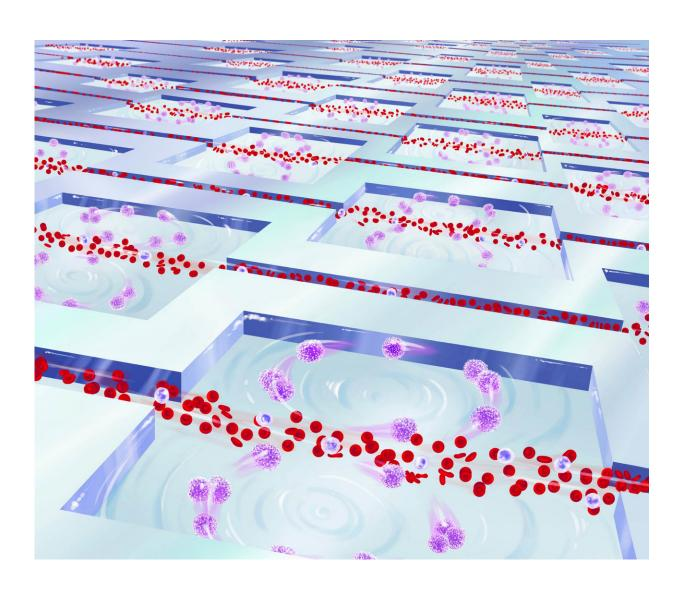
Diagram of how the Vortex Biosciences technology works. A blood sample flows down the micro-channels in the Vortex chip which is designed to form
