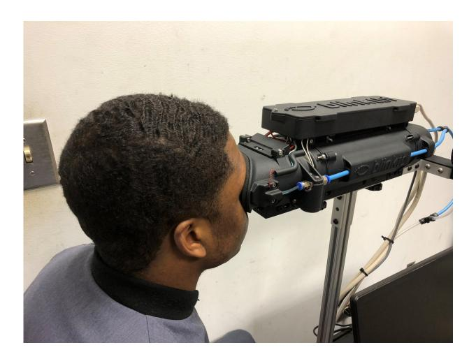
The Blink Reflexometer being used to measure the blink reflex of a cadet at the Citadel. Credit: The Citadel.
