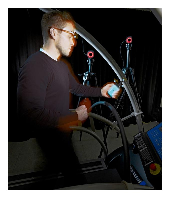
A trial participant performs the visual acuity test with a smartphone while walking on a treadmill. An infrared tracking system monitors the distance between the eyes and the smartphone. Credit: Fraunhofer FKIE
