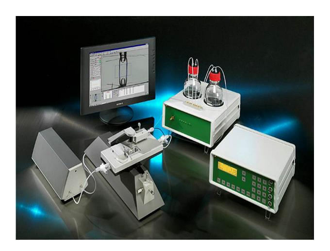
Myograph system used to measure the properties of the arteries under study. On the screen one can see the mesenteric artery of one of the research animal models. Credit: INc-UAB
