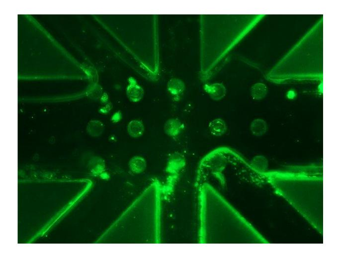
Microscope picture of the microfluidic device developed by Manoj Sharma. The horizontal stripe is the microchannel, which measures 0.2 mm across. The six other stripes are optic fibers that capture the fluourescent light and lead it to a spectrometer. The fifteen dots in the middle are micropillars. Credit: Eindhoven University of Technology
