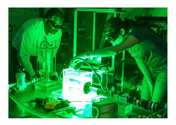
Prasad Dasi, PhD (left) of The Ohio State University College of Engineering tests a 3D-printed aorta in a high-tech simulator that replicates what happens in a specific patient's heart. The experiments allow experts to test different aortic valve replacement options to help doctors prevent complications in the operating room. Credit: The Ohio State University Wexner Medical Center
