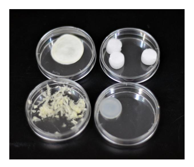
Collagen in different forms could be suitable for different wounds. (Clockwise from top left): Processed collagen made into a patch, foam, hydrated gel, and unstructured form. Credit: NTU Singapore
