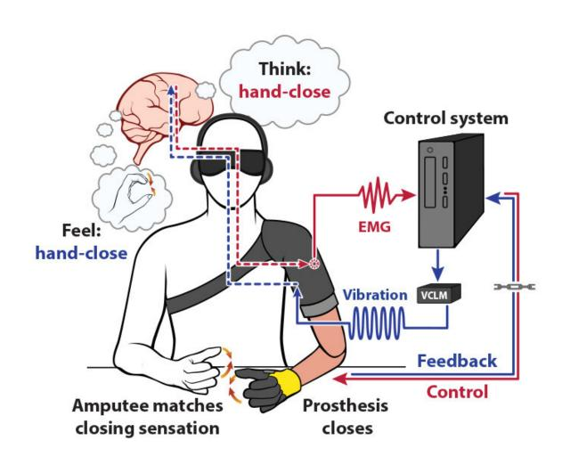
Schematic representation of the movement feedback paired to a real-time, functional prosthetic hand clinically fitted to the participant. Feedback pathways are represented in blue (VCLM, voice coil linear motor). Prosthesis control
