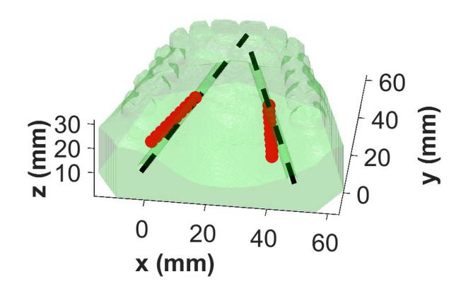
Starfish Engineering LLC has devised an imaging method that works by using contrast in the absorption of light to locate the arteries. The red lines in this graphic show the imaged location of arteries simulated in a 3-D printed mouth phantom. Credit: Purdue University
