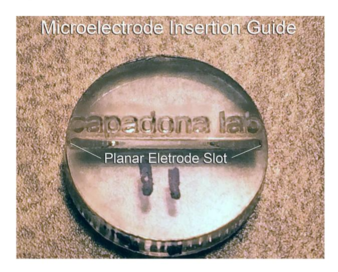
The small, 3-D printed device for inserting soft neural implants. Credit: Case Western Reserve University
