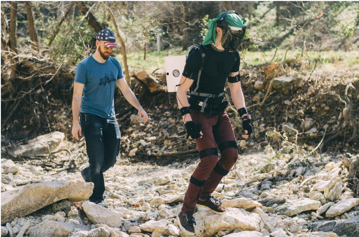
Researchers jerry-rigged a welding mask around an eye tracker -- to shade the infrared eye cameras from sunlight -- and developed new methods to calibrate the eye tracker with a motion-tracking suit to record gaze and full-body kinematics. Credit: Michelle Chiou
