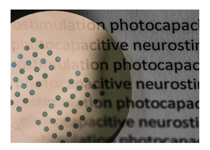
An array of semitransparent organic pixels on top of a ultrathin sheet of gold. The thickness of both the organic islands and the underlying gold is more than one-hundred times thinner than a single neuron. Credit: Thor Balkhed
