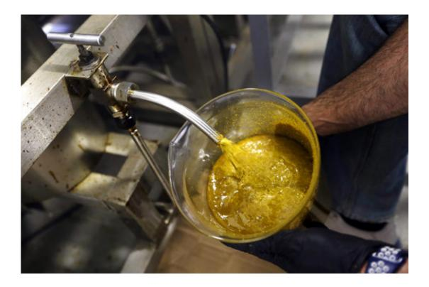
In this April 24, 2018 photo, the first rendering from hemp plants extracted from a super critical CO2 extraction device on its' way to becoming fully refined CBD oil spurts into a large beaker at New Earth Biosciences in Salem, Ore. Applications for state licenses to grow hemp, marijuana's non-intoxicating cousin, have increased more than twentyfold since 2015 and Oregon now ranks No. 2 behind Colorado among the 19 states with hemp cultivation. (AP Photo/Don Ryan)
