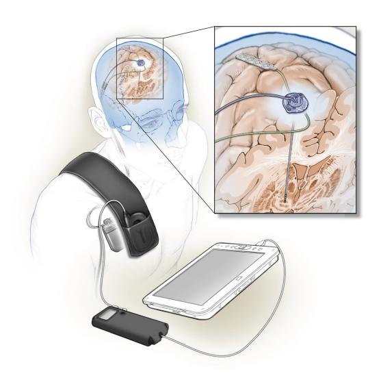
Stimulating and sensing electrodes are implanted in the brain and connect to
