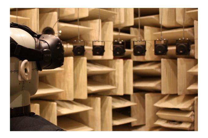
A mannequin wears a VR headset in an anechoic chamber to measure the effects of simulated sound cues from different positions. Credit: Keli Lawrence
