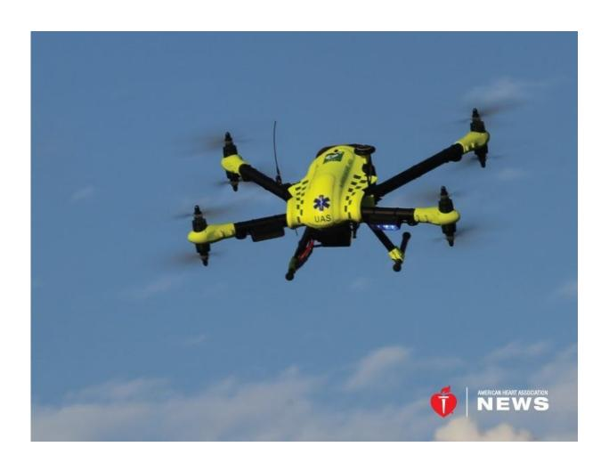
Drones that deliver automated external defibrillators to cardiac arrest victims are being tested in the U.S. and elsewhere. Photo courtesy: The JAMA Network
