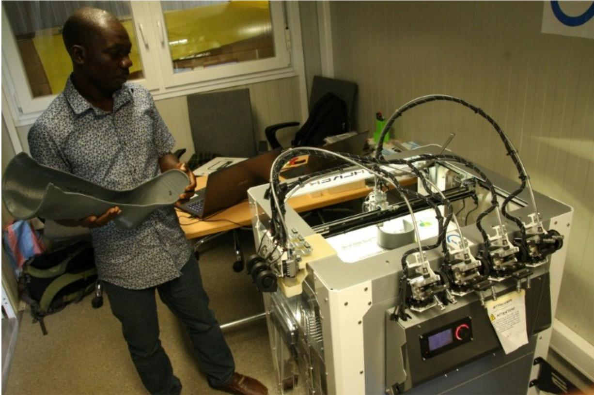
Technician Fabrice Agbelehounko Djodji checks the work of a 3D printer used to produce prosthetic supports at the African Organisation for the Development of Centres for Disabled People in Lome. Making 3D devices locally is expected to cut costs.
