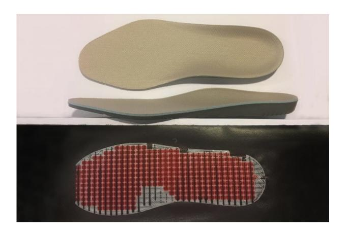
The smart insole can measure gait, activity level and balance and detect a rising temperature which could be a sign of infection. The project is the result of a collaboration between a podiatric surgeon and a neurosurgeon. Credit: Bernard Grisoni, Autonomous ID
