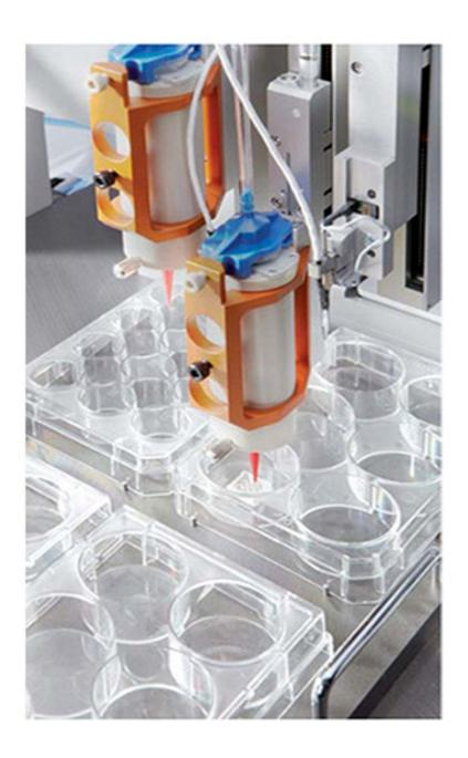
A multichannel bioscaffolder 3D bioprinter that can bioplot the biphasic CPC-
