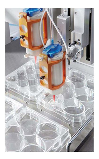
A multichannel bioscaffolder 3D bioprinter that can bioplot the biphasic CPC-
