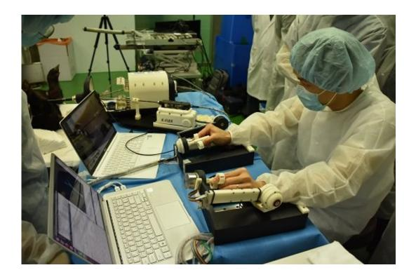
The team conducts a procedure using K-FLEX, flexible endoscopic surgical robot. Credit: KAIST
