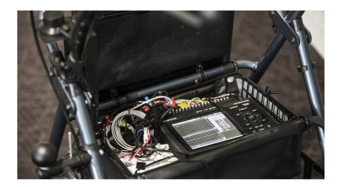
Dr Federico Tartarini collected data from five aged care facilities in the Illawarra, in both warmer and cooler months, using a high-tech, wheeled-walker fitted with temperature, humidity and air velocity sensors. Credit: University of Wollongong
