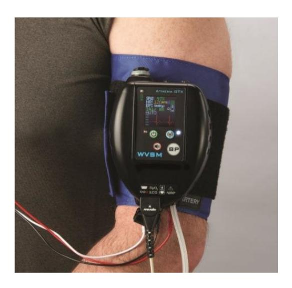
The Wireless Vital Signs Monitor (WVSM). Sponsored by the Office of Naval Research, the WVSM tracks critical health information like heart rate, pulse and blood pressure. It weighs less than a pound and can be carried easily into combat zones or mass-casualty emergency situations. Credit: Athena GTX
