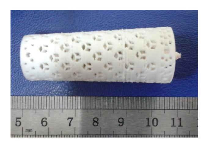
TPU bioresorbable composite implants for testing at the Ilizarov Center. Credit: Tomsk Polytechnic University (TPU)
