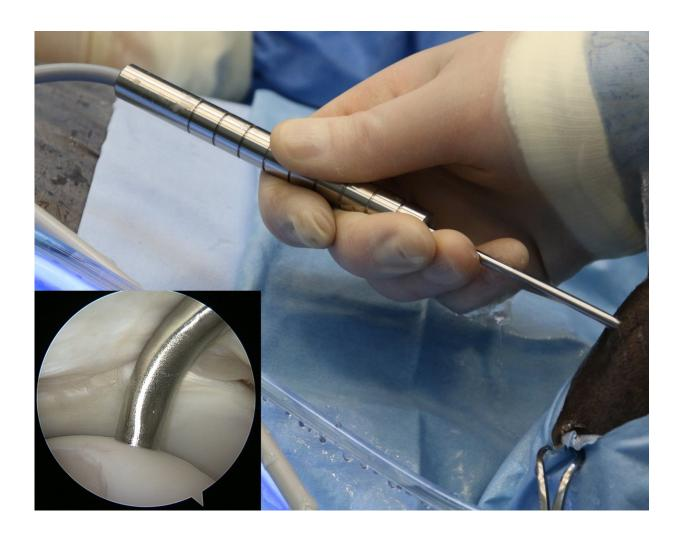
Novel arthroscopic probe.pngPhoto caption: The novel arthroscopic probe in an equine knee joint in vivo with the probe tip in contact with cartilage surface (inset). Credit: University of Eastern Finland
