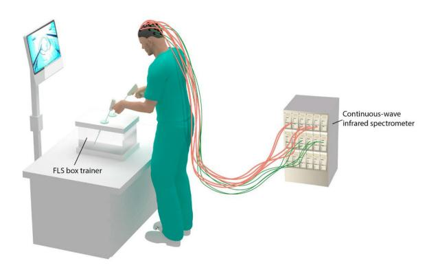
Schematic depicting the FLS box simulator where trainees perform the bimanual dexterity task. A continuous-wave spectrometer is used to measure functional brain activation via raw fNIRS signals in real time. Credit: Nicolás Fernández, Nemani et al., Sci. Adv. 2018; 4: eaat3807
