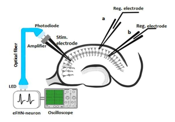
Schematic illustration of an optoelectronic device during the stimulation of synaptic transmission in the mouse hippocampus section. Credit: Lobachevsky University
