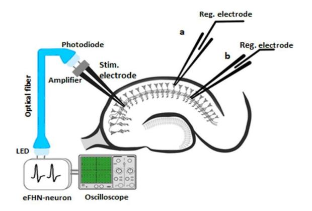
Schematic illustration of an optoelectronic device during the stimulation of synaptic transmission in the mouse hippocampus section. Credit: Lobachevsky University
