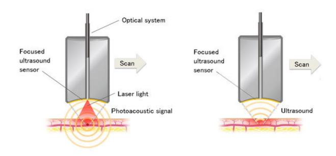
The principle of photoacoustic imaging (left) and ultrasonic imaging (right) using a focused ultrasonic sensor. Credit: Tohoku University
