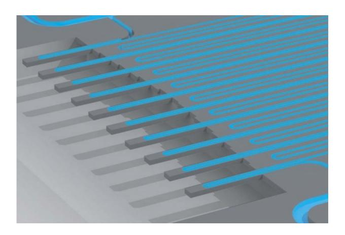
MIT engineers have designed a system that can repeatedly measure cancer cells as they flow through an array of mass sensors. Once the cells reach the end, they are collected for RNA-sequencing. Credit: Massachusetts Institute of Technology
