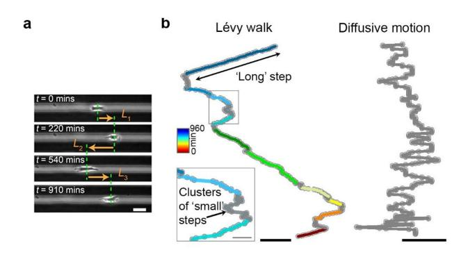
(a) Cell migrating on a linear microtrack. (scale bar =  $20 \mu m$ ) (b) Metastatic cancer cells perform Lévy walk featuring trajectories with clusters of small steps interspersed with rare long strides. In contrast, non-metastatic cells perform diffusive movements with many small steps of similar lengths. Scale bar is  $100 \mu m$  for Lévy trajectory and  $20 \mu m$  for the inset. Credit: (Reproduced from *Nature Communications*).
