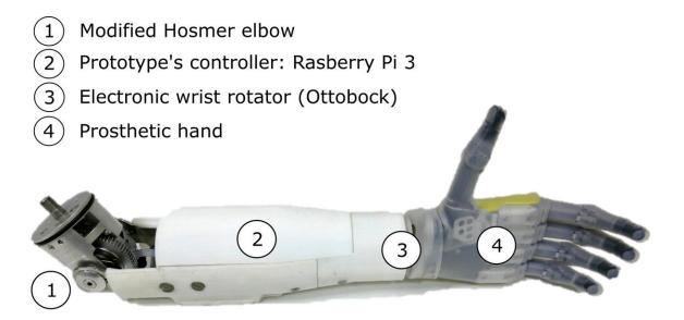
The arm prosthesis prototype used for the experiments, composed of a motorized elbow (1), an electronic wrist rotator (3) and a polydigital hand, the Touch Bionics Robolimb (4). Credit: E. Montalivet 2018.
