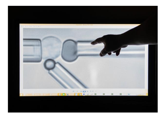
Under the microscope, tiny pipettes tug at living cells to exert forces on their structures, measure those forces and observe the consequences for the cells. Credit: Georgia Tech / Allison Carter
