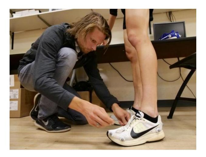
Wouter Hoogkamer places motion sensors on a runner in order to test the biomechanics of the Nike Zoom Vaporfly 4% shoe. Credit: Casey A. Cass/CU Boulder
