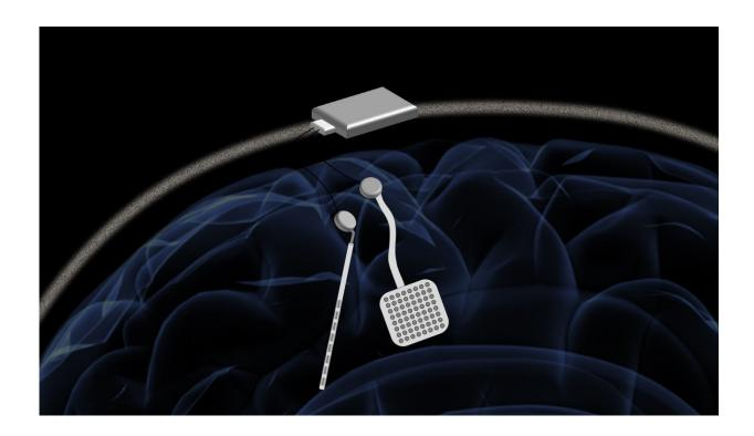
In a proposed device, two of the new chips would be embedded in a chassis located outside the head. Each chip could monitor electrical activity from 64 electrodes located into the brain while simultaneously delivering electrical stimulation to prevent unwanted seizures or tremors. Credit: Rikky Muller, UC Berkeley
