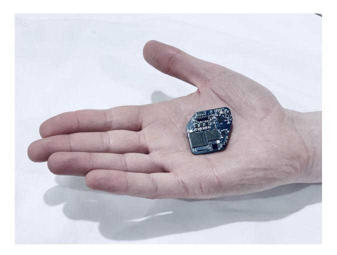
The WAND chip is designed with custom integrated circuits that can record the full signal from both subtle brain waves and strong electrical pulses delivered by the stimulator. Credit: Rikky Muller, UC Berkeley
