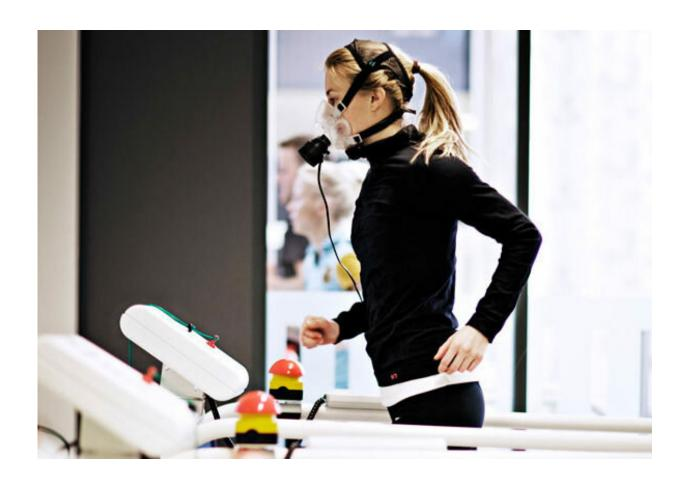
Researchers use a treadmill and a special mask to measure a person's maximum oxygen uptake, which is considered an important measure of fitness. Credit: Geir Mogen/NTNU
