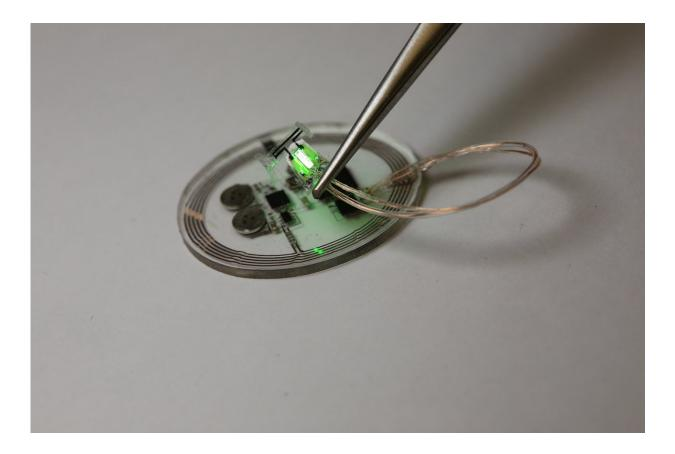
A soft, fully wireless bioelectronic device for automated closed-loop optogenetic neuromodulation of bladder function. Credit: Sang Min Won
