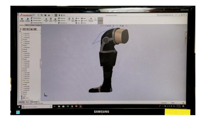
The proposed brace is the first lower extremity device designed to correct alignment or provide support using soft muscle-like "smart materials" that contract in response to electric current. Credit: University of Delaware
