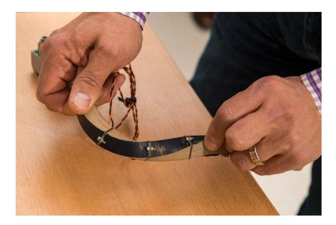
The artificial muscle shown is flexible and uses "smart materials" to mimic the function of the body's skeletal muscle. Incorporated into a wearable device, the artificial muscle can help researchers increase the wearer's degrees of freedom in movement. Credit: University of Delaware
