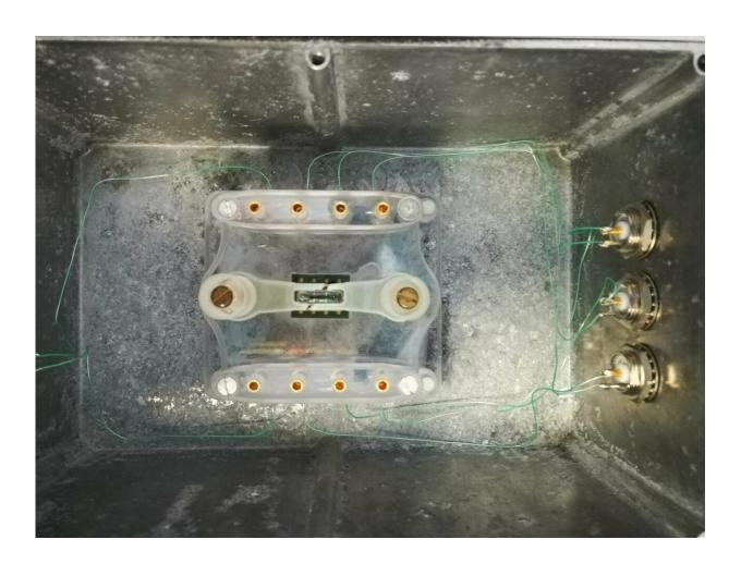
Chip in the box, shows how the silicon chip is installed in the box in which it will be introduced into the incubator. Credit: University of Seville
