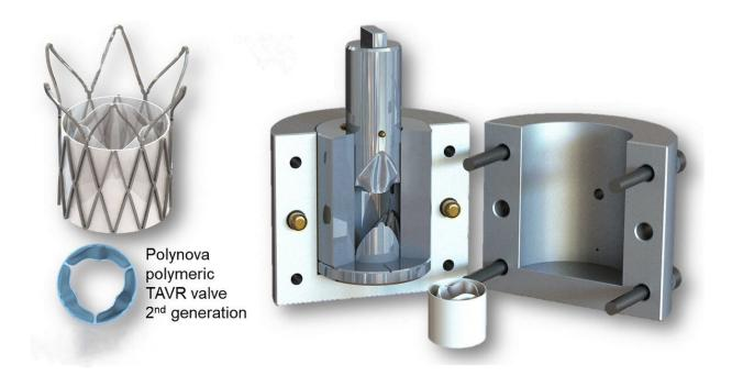
New aortic heart valve made of polymers instead of animal tissues (left). Compression injection mold used to make new valve allows mass production of valves at reduced cost (right). Credit: Rotman, et al. Ann Biomed Eng-Jan 2019: Springer Nature
