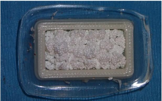
3D-printed bioreactors filled with autologous bone (top) or a synthetic graft (bottom) are key components of a new technique to grow custom-fit bone
