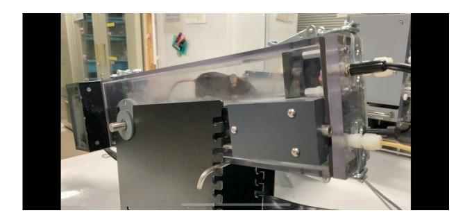
During the experiment, mice with induced heart failure and in the control group were placed in this device to measure their exercise abilities.
