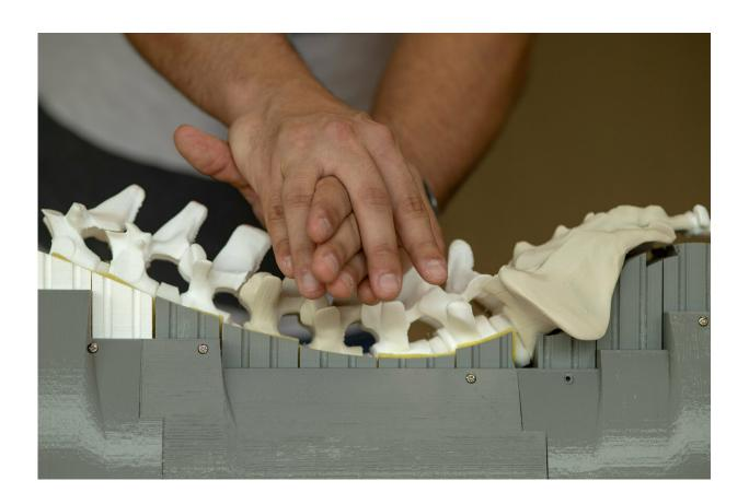
Using smart foam sensors, SpinalLog measures the pressure being applied to the spine by the student's hand or fingers during a simulated assessment. Credit: Sarah Fisher, University of Melbourne
