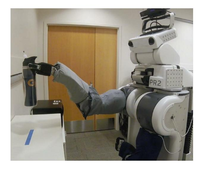
Showing its capabilities as a body surrogate, a PR2 controlled remotely by an individual with profound motor deficits picks up a cup in a research laboratory at the Georgia Institute of Technology. Credit: Phillip Grice, Georgia Tech
