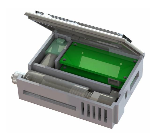
Inside the wearable device, the blood pump sits in the upper left corner while the heparin injector runs the length of the near side of the box. The green circuit boards control the blood pump, heparin injector and provide display data. Credit: Tae Hyun Kim
