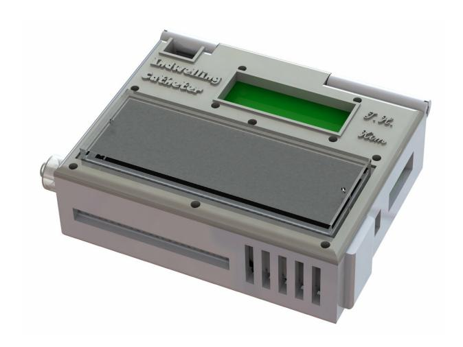
The wearable device measures roughly  $2 \times 2.75 \times 1$  inches, with the cancer-cell-capturing chip mounted on top. The catheter connecting to the patient runs through the hole in the top left corner. Credit: Tae Hyun Kim
