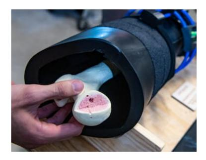
Rice engineering students have created a device to simplify the insertion of screws that secure metal rods to fractured bones in limbs. The device, when secured on the leg of a patient, uses magnetic elements in the rod to guide proper placement of the screws. Credit: Jeff Fitlow
