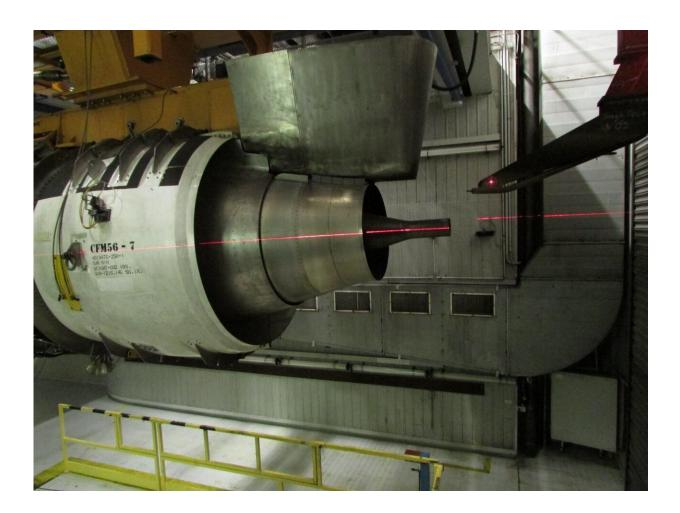
Close-up of the turbine engine at the testing facility with the aerosol sampling probe in place (right). Credit: University of Bern /SR Technics Switzerland AG
