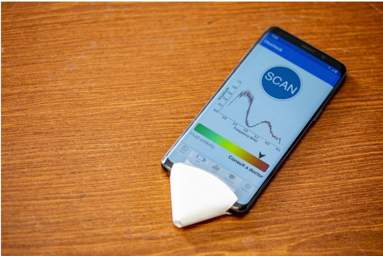
University of Washington researchers have created a new smartphone app that can detect fluid behind the eardrum by simply using a piece of paper and a smartphone's microphone and speaker. Credit: Dennis Wise/University of Washington]
