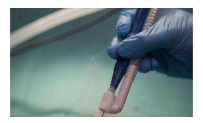
Flue gas created by an electric knife is fed directly into the measurement system. Credit: Antti Roine
