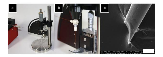
A hollow micro-needle and applicator. Credit: Pim Schipper
