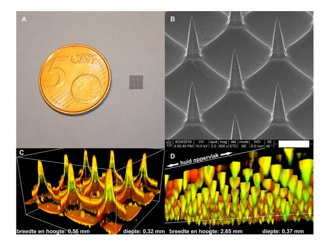
Upperleft: array with solid micro-needles and a nickel. Upperright: an enlarged picture of the micro-needles. Lower left: the same micro-needles but coated. Lower right: an image of the skin after the application and removal of coated micro-needles. Credit: Pim Schipper
